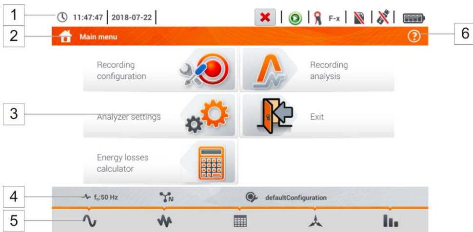
Fig. 5.2 Main elements of the recorder screen
